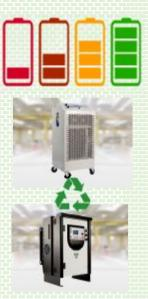
We program the BLT for a TEST5 with 1 cycle, with the battery status to be plenty (all 5 leds inside the battery symbol are ON) and the AhB is equal to the nominal C5 capacity: in this way the BLT will start with a Discharge. Since the charging current is 1/30 C5, it is important to Set on the BLT. MaxCT to 40h and MinCT to 36h so that the charger have enough time to fill the battery.
